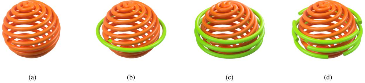
Fig. 2: Design evolution of the proposed antenna, showing (a) the base 4 arm, 1.5 turn folded spherical folded helix, (b) addition of a parasitic loop around the antenna to reduce axial ratio, (c) multiple parasitic loops, and (d) the introduction of cuts in the parasitic loops for tuning of the resonant frequency.
